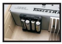
The CI-50 uses AA batteries. Easy to find and easy to replace. The AA batteries in the CI-50 will keep it operating for more than 80 hours.
