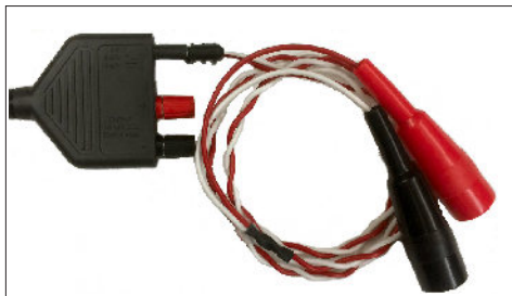
Twisted Wire Cable Connected to Power Cable
